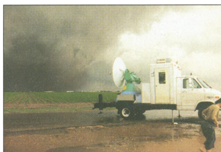
Fig. 2. DOW mobile radar with Dimmitt, Texas, tornado in background. The range to the edge of the cone-shaped visible debris shield around the tornado is approximately 2.5 km.
