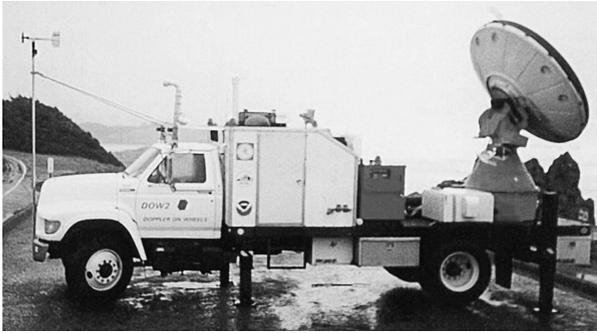
FIG. 2. A DOW mobile radar. The 2.44-m-diameter antenna produces a  $0.93^\circ$  beam and can scan at speeds up to  $60^\circ \text{ s}^{-1}$ . The leveling and stabilization system provides a stable platform in high winds that can be leveled with an accuracy of about  $0.2^\circ$  within about 40 s. The operator cabin to the rear of the truck cab encloses transmitting, receiving, signal processing, navigational, antenna control, and other hardware.
