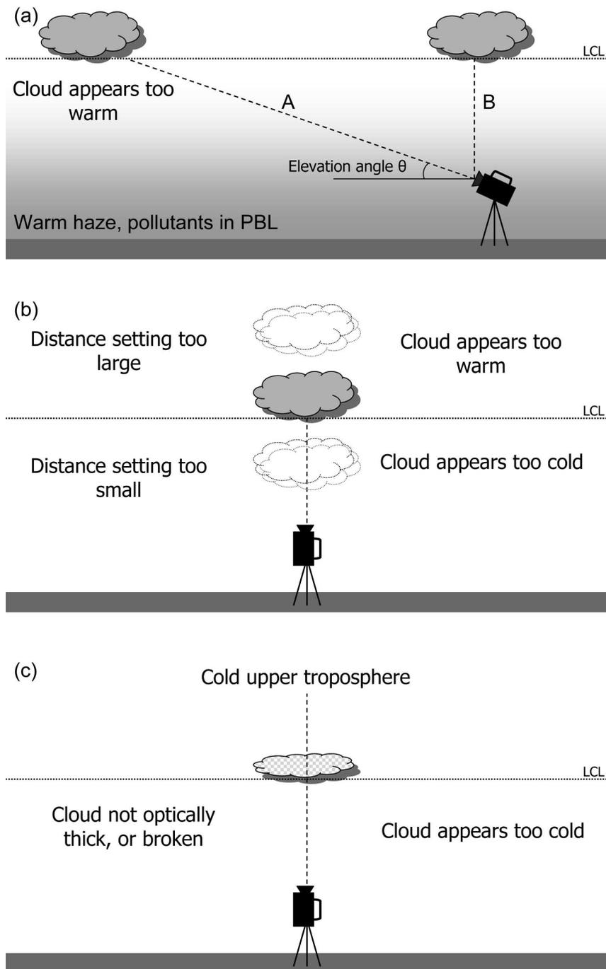
FIG. 5. Explanations of erroneous cloud temperature readings by the infrared camera during the atmospheric transmissivity study. (a) Changes with elevation angle: A cloud viewed via line-of-sight A will appear warmer than a cloud viewed via line-of-sight B. (b) Changes with camera distance setting. (c) Changes with cloud opacity/optical thickness. In our atmospheric transmissivity study, the effect described in (a) dominated the effects described in (b) and (c).
