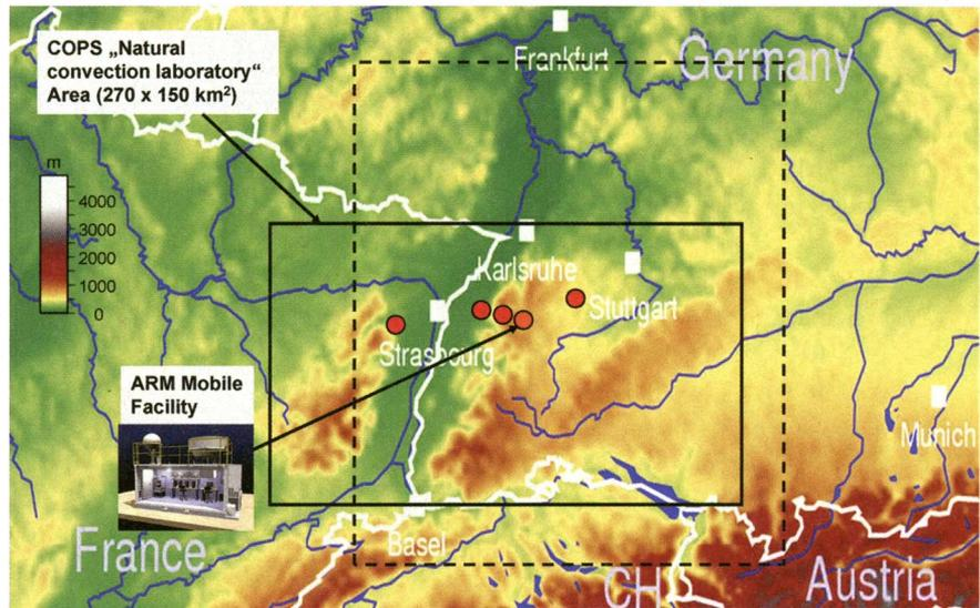
**FIG. 2.** Solid black line: the COPS region. Dashed black line: validation box shown in Fig. 1. Red/orange circles: locations of five Supersites where a synergy of remote-sensing systems was deployed. The orange circle represents the Atmospheric Radiation Measurement Program Mobile Facility (AMF).
