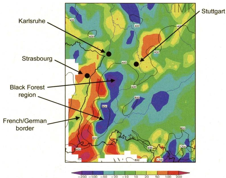
**FIG. 1. Difference (mm) between predicted and observed precipitation in the Black Forest region for August 2004 using the COSMO model of the DWD with a grid resolution of 7 km, confirming the windward/lee problem. The thin black lines indicate the topography. The mean prevailing wind is from the west. The locations of major cities and the French/German and German/Swiss borders are also shown. (Courtesy of L. Gantner, IMK, Karlsruhe, Germany.)**
