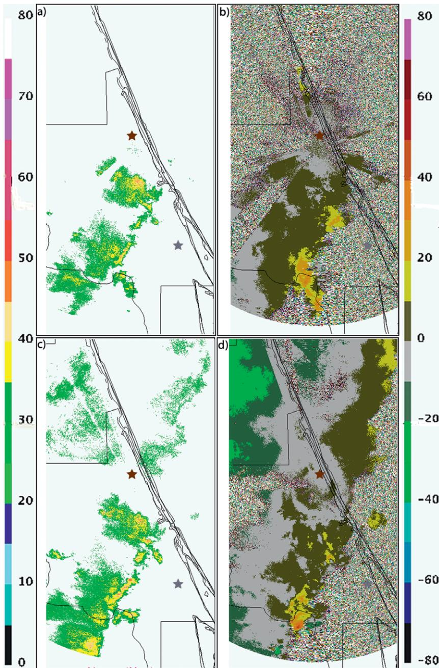
**FIG. 10.** (left) DOW-6 base reflectivity (dBZ; shaded) and (right) base radial velocity (kt) at 2230 UTC 20 May 2015, during IOP9, for the (a),(b) 1° and (c),(d) 5° elevation scans. The stippled areas in (b) and (d) are artifacts of the DOW-6 radial velocity scans and should be ignored. As in Fig. 9, the IOP9 scanning location (Fig. 3; Table 2) and Edgewater are marked with brown and gray stars, respectively.
