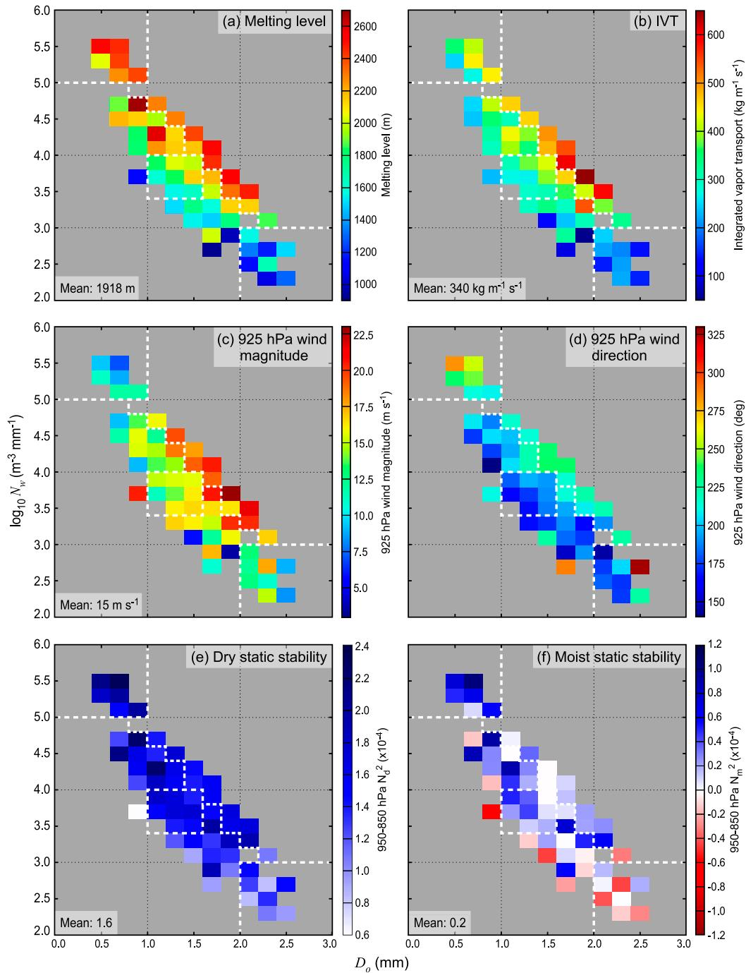
FIG. 5. Average synoptic environmental parameters calculated at the NARR grid point closest to NPOL. (a) Melting level (m), (b) IVT ( $\text{kg m}^{-1} \text{s}^{-1}$ ), (c) 925-hPa wind speed ( $\text{m s}^{-1}$ ), (d) 925-hPa wind direction ( $^{\circ}$ ), (e) dry Brunt-Väisälä frequency ( $N_d^2$ ), and (f) moist Brunt-Väisälä frequency ( $N_m^2$ ). The data are binned by the Prairie Creek 3-h DSD as in Fig. 3b. The white dashed lines are as in Fig. 3.
