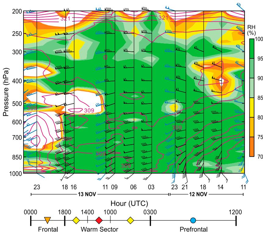
FIG. 10. Time–height cross section of soundings launched during the 12–13 Nov 2015 case study. Black lines and wind barbs (kt; 1 kt = 0.51 m s<sup>-1</sup>) denote soundings launched from NPOL. Blue lines and wind barbs (kt) denote soundings launched from Quillayute (Fig. 2). Red contours denote potential temperature  $\theta$ . Colored contours denote relative humidity (%). Figure provided by Paul Ciesielski.
