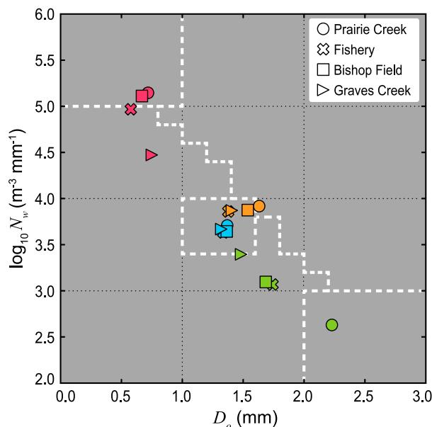
FIG. 7. Scatterplot of the overall  $D_o$  vs  $\log_{10}(N_w)$  relationship for four of the ground sites. Each point represents the combined DSD for the times that Prairie Creek falls into each of the four DSD regimes. The colors correspond to the regimes in Fig. 6: most frequent (blue), small drops (red), large drops (green), and heavy rain (orange).
