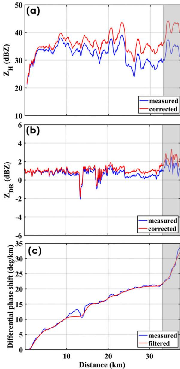
FIG. 4. Ray profiles of measured (blue line) and attenuation-corrected (red line) (a)  $Z_H$ , (b)  $Z_{DR}$ , and (c)  $\phi_{DP}$  for the 8 Dec 2015 event at 0238 UTC. The gray regions represent the bright band.
