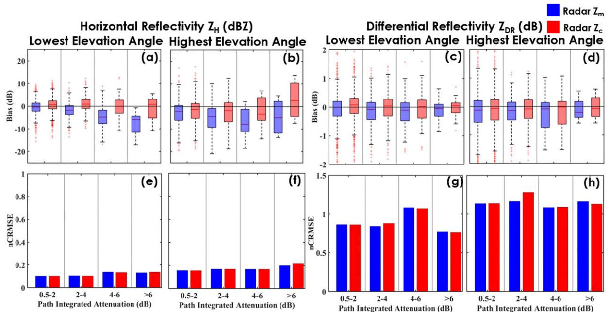
FIG. 5. Bias and nCRMSE bulk error statistics of measured (blue bars) and attenuation-corrected (red bars) (a),(b),(e),(f) horizontal reflectivity  $Z_H$  and (c),(d),(g),(h) differential reflectivity  $Z_{DR}$  parameters vs PIA. Results are presented for the lowest elevation angles in (a), (c), (e), and (g) and the highest elevation angles in (b), (d), (f), and (h).
