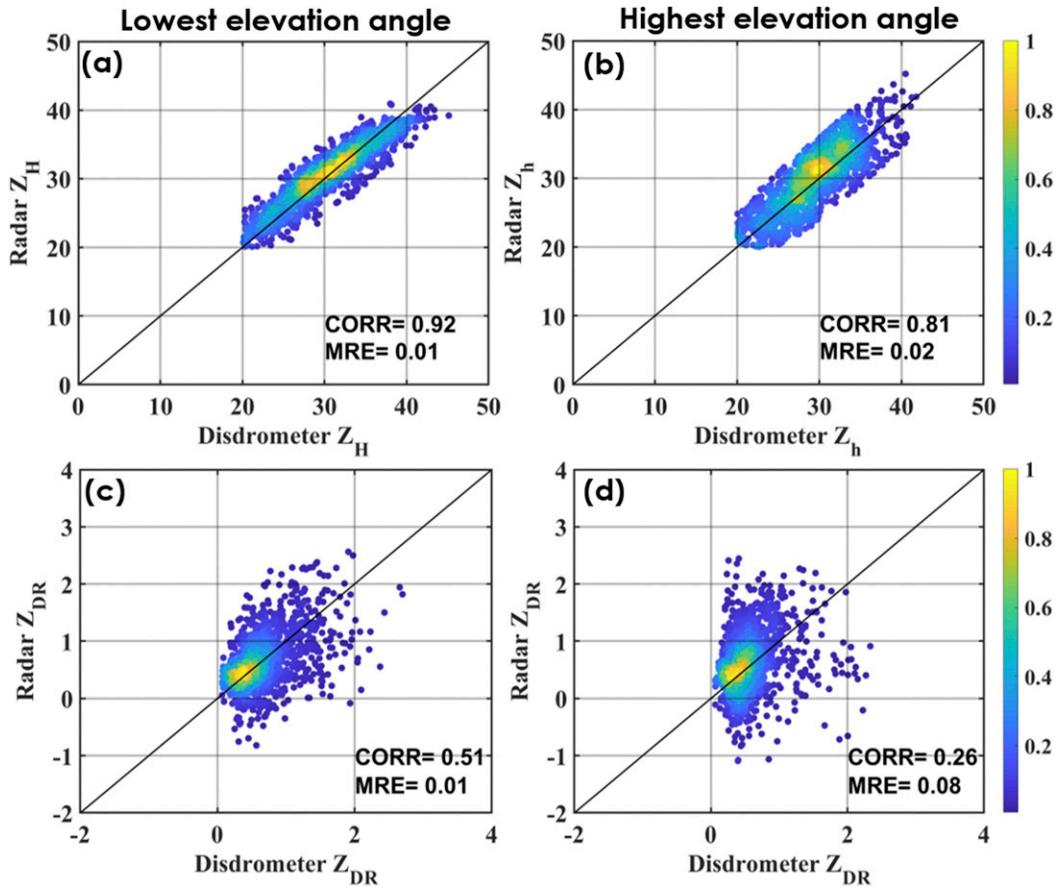
FIG. 2. Attenuation-corrected (a),(b) horizontal reflectivity  $Z_H$  and (c),(d) differential reflectivity  $Z_{DR}$  (dB) comparison for the (left) lowest elevation angle and (right) highest elevation angle between the disdrometer and DOW for the closest APU disdrometers.
