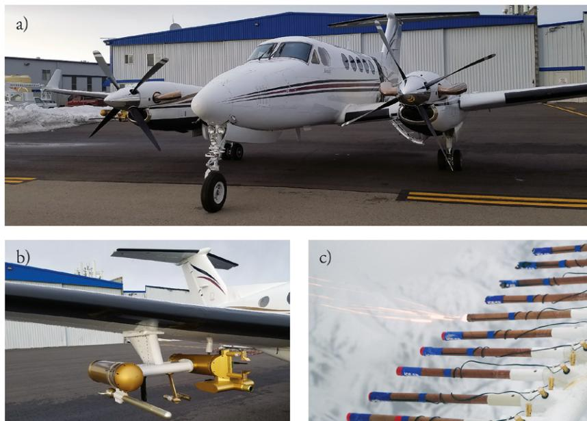
**FIG. 2.** Photos of (a) the WMI seeding aircraft, with close-ups of (b) instruments mounted under the wing and (c) the wing-mounted BIP flare rack with one BIP flare lit during seeding. (Photos courtesy of A. Brainard, WMI.)
