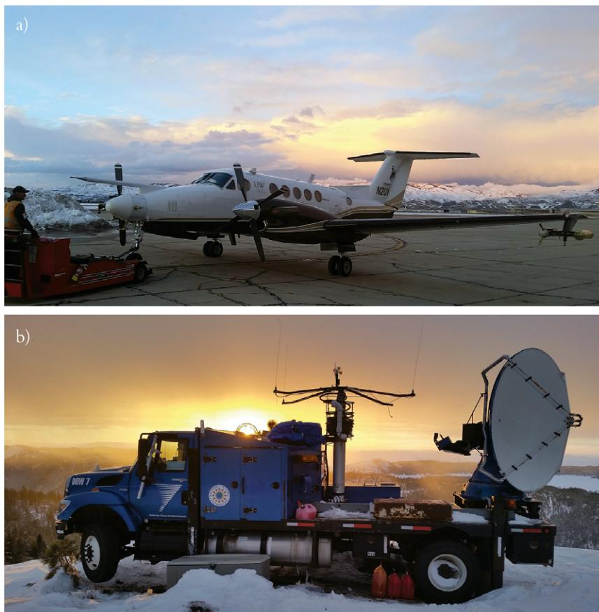
**FIG. 1. Photos of (a) the UWKA aircraft (courtesy L. Oolman, University of Wyoming) and (b) the DOW-7 radar located at Packer John at sunset (courtesy J. Aikins, University of Colorado Boulder).**
