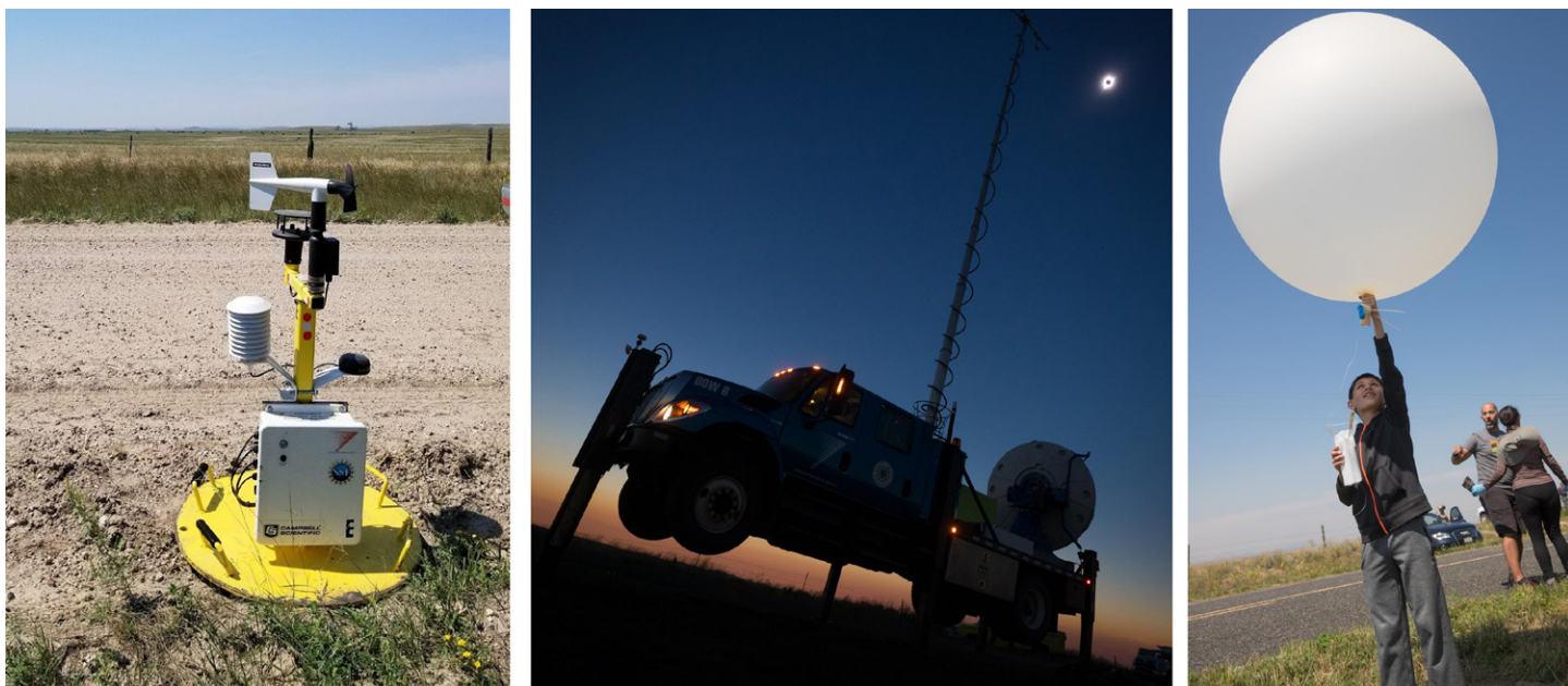
FIG. 4. FARM DOW and micronet instruments. (left) Pod E deployed in an open area before totality; (center) DOW scanning during totality, with the sun at the time of totality visible at the top right; and (right) balloon sounding being launched before totality.
