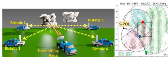
Figure 17. (left) Schematic mobile bistatic network with four receiving antennas and one transmitting radar. The transmitting radar is, in this example, a DOW or SOW, but can be a stationary radar (e.g., S-POL). The four receiving antennas are on the back of pickup trucks, but can be deployed similarly to Pods. The transmitting and receiving radars can be moved like MMs to optimize coverage and vector wind retrievals as phenomena move/evolve. As the DOW/SOW transmits and scans, the pulses in its narrow radar beam (orange arrow) are scattered from hydrometeors, dust, etc. Some of that scattered energy (dashed yellow arrows) is received by the passive antennas, as well as the by the DOW/SOW antenna (dashed orange arrow). Three-dimensional vector wind fields are calculated from these various Doppler measurements. (right) An example of vector wind retrievals from a bistatic network. In this example, there was one transmitting radar (S-POL) and three bistatic receivers (solid squares). The colored vectors depict the retrievals using data from the north (red), central (blue), and southern (green) bistatic receivers. Arcs depict the bistatic dual-Doppler lobes with the transmitting radar. The square outline encloses an overdetermined analysis domain. (Image adapted from Satoh and Wurman 2003).
