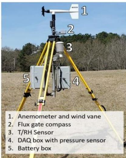
1. Anemometer and wind vane
